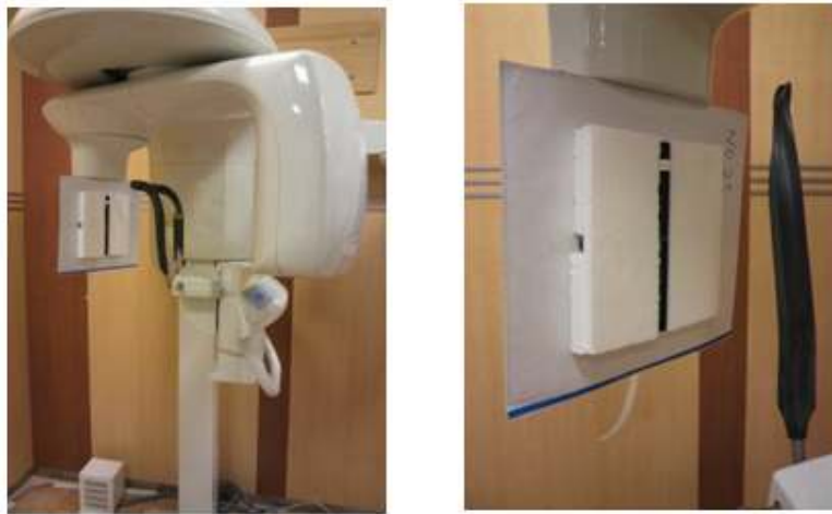
Figure 3 Film packet with dosimeter on CBCT unit for dose measurement (Endo A et al 3) Figure 2を元に著者が一部手を加え作成した)
